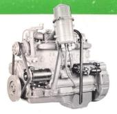
The Mack END 673E is a naturally aspirated, four cycle, open chamber, overhead valve designed engine. Uniform cooling is achieved through directed water flow. Fully counter-balanced, induction case-hardened crankshaft with cool running hollow crank pins and a viscous type vibration damper are used.
