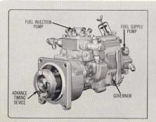
Advance timing unit, single plunger type fuel injection pump, governor and fuel supply pump sealed assembly is driven from the timing gears. The flange mounted assembly is independent of engine valve mechanism which makes for ease of maintenance. Retardation is provided in coasting by complete fuel shut-off. Exclusive automatic injection timing device assures exceptionally smooth running and easy starting.
