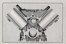
Coolant distribution is exceptionally uniform with directed feed to the points where combustion heat effects are greater. Three cylinder sleeve o-ring seals are used. Recessed into the block rather than the sleeve, they provide longer seal life and a weight-saving sleeve design.
