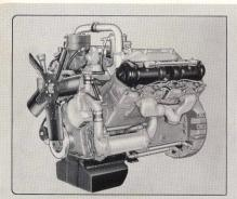
Large aluminum inlet manifolds assure high breathing for utmost volumetric efficiency. Exhaust manifolds are designed to permit rapid expulsion of the hot gases. New pressed steel pan design assures lubrication even on the severest grades. The oil pump located in the oil sump affords quick engine lubrication upon starting.
