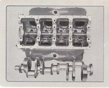
The accurate cylinder block casting is a rigid structure with five main and camshaft bearings supported in husky bulkheads. Mack crankshaft is integrally balance-compensated for V8 operation. The skew drilled connecting rod lube oil passages are located for ideal oil feed relation to the bearing.
