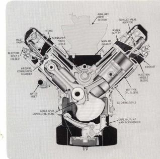
This, combined with an improved single plunger type fuel injection system, operating at moderate pressure, produces high thermal efficiency and therefore sustained economy through a broad range of useful speeds. Smooth and flexible operation results from the automatically controlled injection timing device for best results at all engine speeds. In addition, it assures quick starting, even at low temperature.
