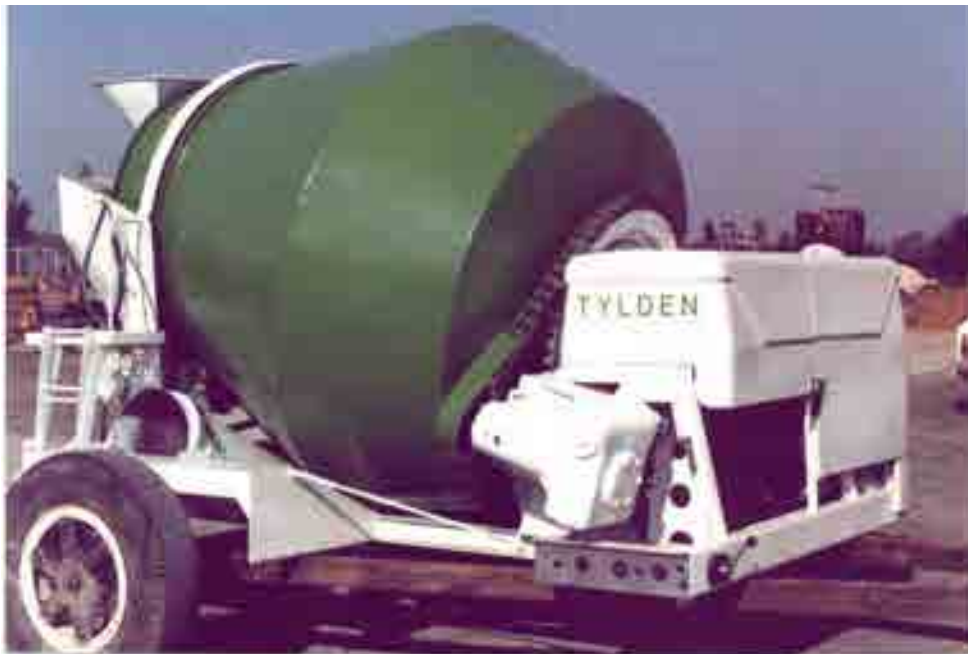
One of the first Tylden mixers built with modified Fowler Rex G parts.
