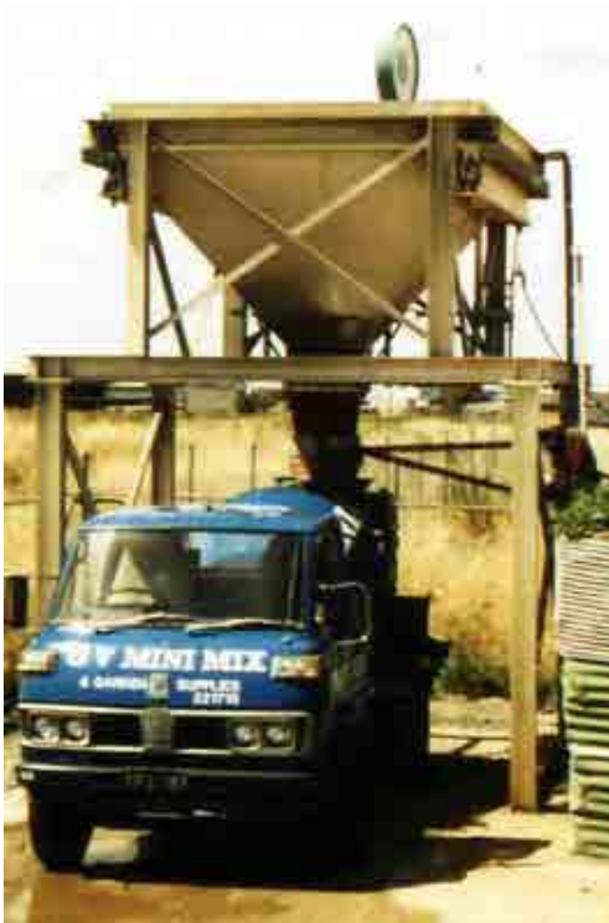
An ME Batcher built for GV Mini Mix at Shepparton. These were very simple and cheap material weigh hoppers for weighing sand and aggregate and bag cement. We also built a 6m3 one and a RK series with a built in cement weigh hopper for bulk cement
