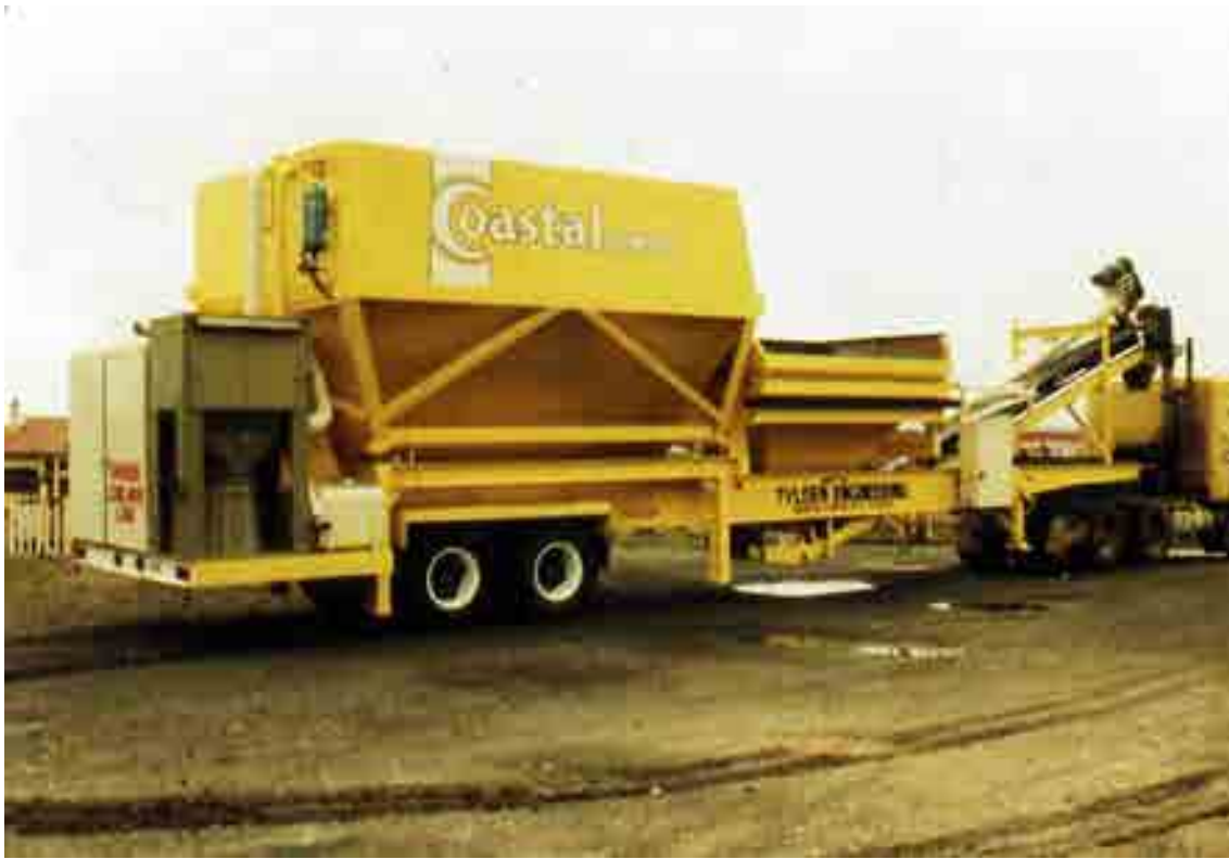
PM series Fully Mobile Batching Plant. This plant was an improvement on our first one as it did not need a crane. It did however need a two level site.
