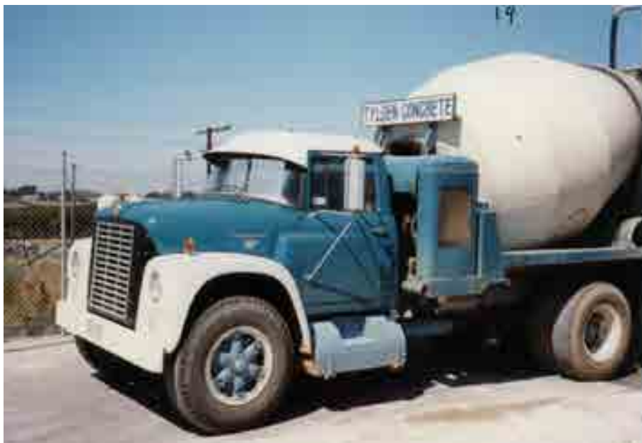
One of the first Tylden mixers built with modified Fowler Rex G parts.
