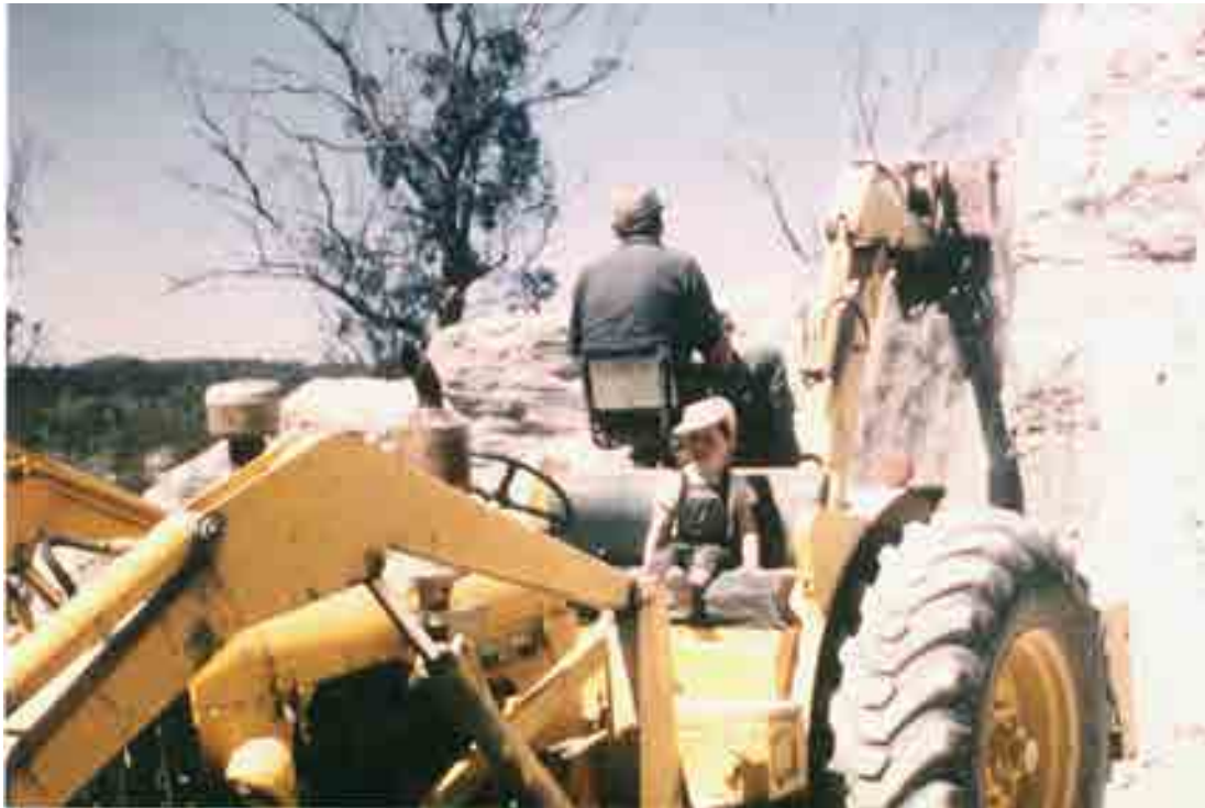
The new Chamberlain Mark 11 powered by 470D Diesel with Superlift loader and backhoe. Pulling down packed battery sand for easy loading at Wattle Gully goldmine. My little helper is Rod..1968
