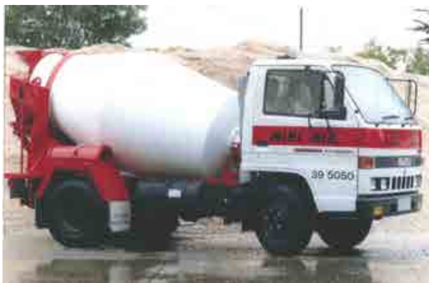
Tylden Midget 1.6 m3 Mixer. The first model we sent to the USA. Later units sent were larger capacity
