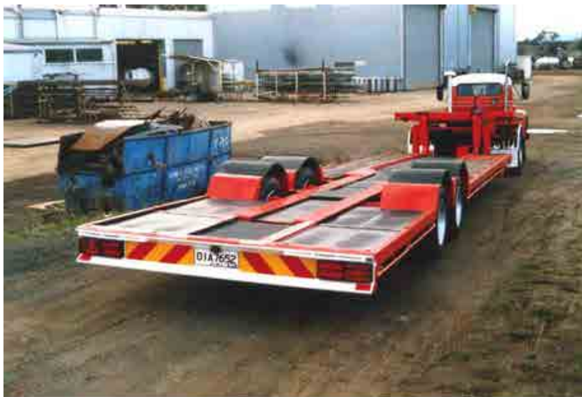
5 July we finish fitting new axles and air suspension to our old drop deck trailer. We build a sleeper box with twin beds, 2 hot plates, microwave, fridge, toilet, TV, running water and own power supply
