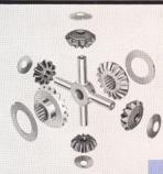
Self lubricating, four-pinion type differential provides a greater distribution of stress. Extra strong gears assure long life. Mack Designed and manufactured, the Dual Reduction axle is a single speed type with two ratio steps in the carrier gears.
